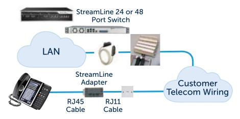
Simply deploy StreamLine by connecting it directly to your LAN and adding a StreamLine adapter to each endpoint.
